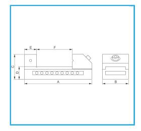
Overall sizes Opening Jaw height Accuracy Gross weight EAN Code 100 x 245 x 90h mm 125 mm g 45 mm 0,005 mm 9,30 kg 8012667204211
